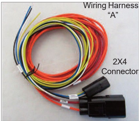
Harness "A" connects into connector "B" from the throttle body mounted ECU. See figure 8
